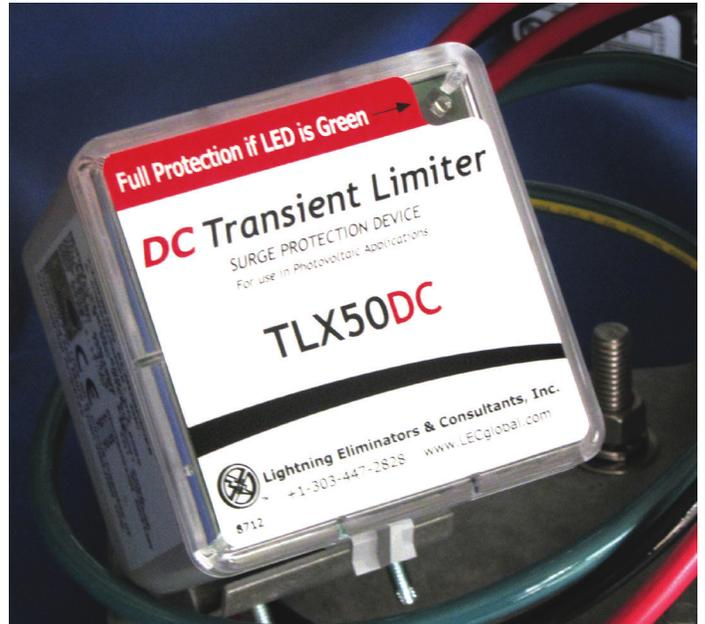
The TLX50 line can be used **indoors or outdoors**, mounted to the electrical panel through a direct nipple connection. The LED status indicator provides a quick visual diagnostic.
