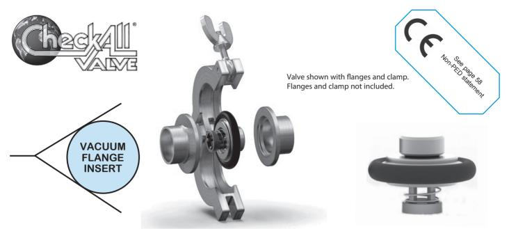
The **Vacuum Flange Insert (VI)** valve is designed to fit between ISO/NW/KF/QF vacuum flanges designed in accordance with DIN 28403, DIN 28404, ISO 1609, and ISO 2861. It is both a centering ring and a check valve. The compact design requires no additional space in the line. Its size makes it extremely economical when compared to full-bodied valves.
