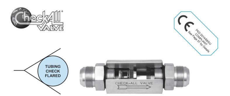
The **Tubing Check Valve-Flared (TF)** is a three-piece constructed check valve with 37° flared end fittings that conform to SAE J514 & ISO 8434-2 . These valves are designed for maximum flow with minimal pressure drop. The TF valve can also be used as a low pressure relief valve or vacuum breaker by using the desired spring settings.
