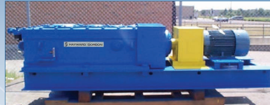
Right Angle Drive model LBX-150 with a high speed flexible fluid coupling.
