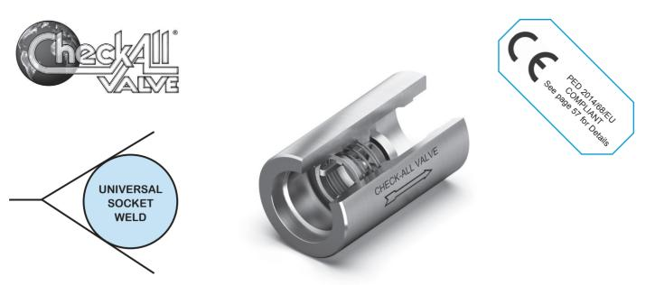
The **Universal Socket Weld (US)** check valve is a one piece body machined from bar stock with socket weld ends and is designed for minimum pressure drop. It carries rugged, dependable Check-All<sup>®</sup> trim and there are wide variety of seat materials and cracking pressures to choose from. The socket ends are machined to ASME/ANSI B16.11 dimensions. The US valve can also be used as a low pressure relief valve or vacuum breaker by using the desired spring settings.
