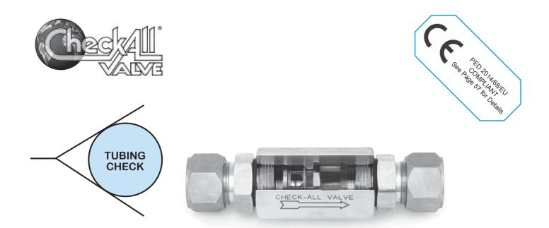
The **Tubing Check (TV)** valve is constructed with compression tube fittings (flareless) and is designed for a minimum pressure drop. The valves are furnished complete with ferrules and nuts. The TV valve can also be used as a low pressure relief valve or vacuum breaker by using the desired spring settings.
