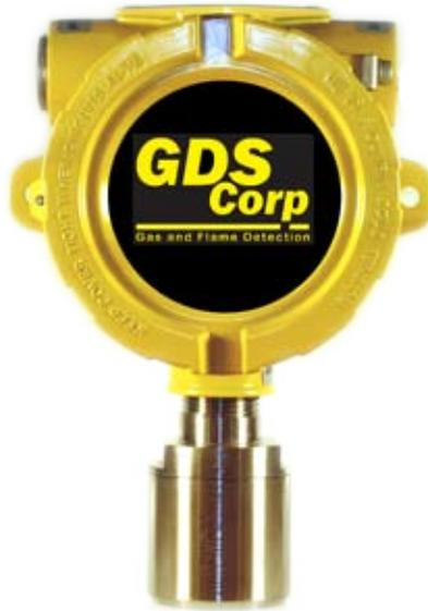
The GDS-50 is a three-wire remote sensor transmitter designed specifically to detect combustible hydrocarbons or carbon dioxide gas. The GDS-50 sensor transmitter 4-20mA output is compatible with the *C1 Protector*, *C2 Protector*, *C2 Quad Protector* or *C64 Protector* Controllers, the *GASMAX II* or *GASMAX CX* gas monitors or any other device with a 4-20mA input and built-in calibration capability.
