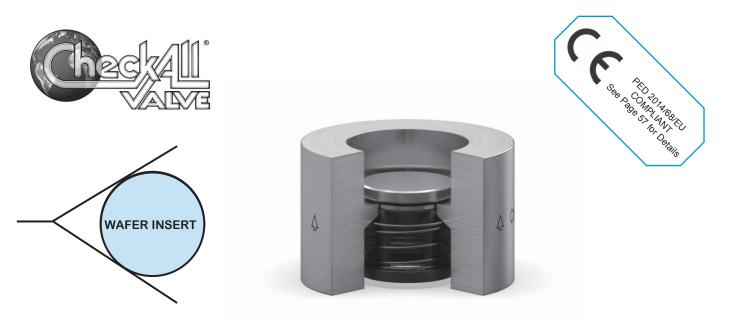
The **Wafer Insert (WV)** valve is designed to fit between two mating ANSI flanges. Two gaskets are required, instead of the one normally used in a flanged joint. The "drop in" valve body fits inside the bolt circle for quick installation and removal in rigid piping applications where the use of the F1, F6, or FP (see our Flange Insert series on page 5) is not practical. Many valves in this series can meet API 594 and/or B16.34 requirements. Consult the factory for more information.
